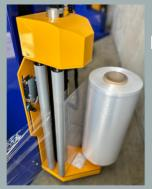
High efficiency mechanical brake carriage with spring handle
